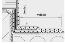
EVALASTIC® VSKA tapes are produced with a non-coated welding edge on both sides or on one side. Thus, a homogeneous welding of the EVALASTIC® VSKA tapes to the roof sealing is guaranteed.
