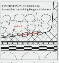
Secure flashing against the waterproofing
